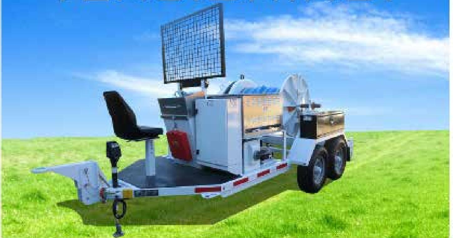
*THE NEWLY DESIGNED DPT40E IS POWERED BY A REGENERATIVE ELECTRIC MOTOR, ELIMINATING THE NEED FOR DIESEL AND HYDRAULIC OIL.*
