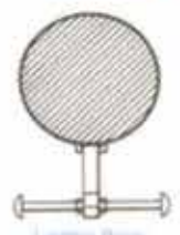
Ladder Pegs Pegs are Aligned for Easier Climbing
